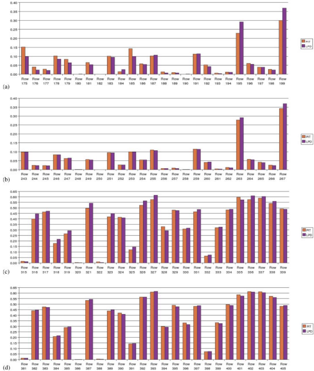
Figure 11. Comparison of aerosol deposition data computed with LPD and PIT methods for two different objects and different number of particles. X-axis corresponds to different aerosol release scenarios; Y-axis shows the number of particles that hit the object divided by the total number of particles released: (a) object 1, N_p = 10^3 ; (b) object 1, N_p = 10^5 ; (c) object 2, N_p = 10^3 ; and (d) object 2, N_p = 10^5 .
